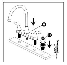
Insert Faucet Body (A) and Sprayer Holder (D) through sink deck.
