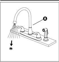
Remove faucet aerator from Faucet Body (A). Rotate counterclockwise to loosen. Turn on faucet and check for leaks. Replace faucet aerator.
