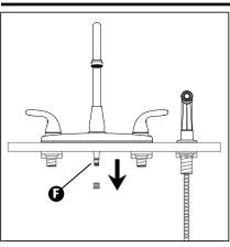
Remove cover from bottom of Sprayer Hose Water Supply **f**.
