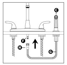
Connect Sprayer Hose **G** by pushing Sprayer Hose Water Supply Connector **1** onto faucet's Sprayer Hose Water Supply **5**. You will hear an audible "click" when the connection is made.
