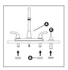
Secure Faucet Body A to sink deck by attaching Faucet Quick Connect Mounts B to hot and cold supply studs. Rotate Faucet Quick Connect Mounts Clockwise to tighten. Follow same process if installing optional Sprayer Holder D.
