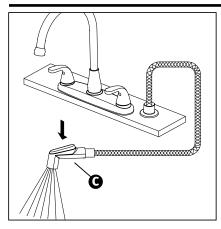
While faucet is on, check water flow from Sprayer **G**. Check for and fix any leaks.
