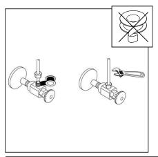
Connect hot and cold supply lines to hot and cold supply valves. DO NOT use plumber's tape if a rubber washer is seated in the Supply Line's connector.
