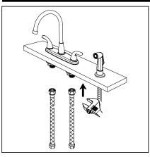
Attach hot and cold supply lines to faucet supply line studs.
