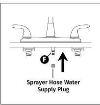
6b If you're not installing the Sprayer **©**, install the Spray Hose Water Supply Plug **6**.
