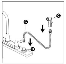
Connect Sprayer Hose G to Sprayer C and insert Sprayer Hose through Sprayer Holder D.
