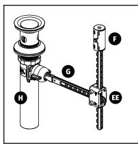
Push corresponding buttons on Rod Holder (1) to adjust position of Clevis (2) and Pivot Rod (3) as required for Pop-Up Drain Assembly **1** to function correctly and seal the drain.
