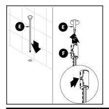
Insert Drain Rod (5) through Faucet Body (A) and attach to Clevis (5).
