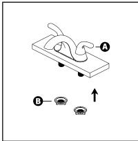
2 Secure Faucet Body (A) to sink deck by attaching Quick Connect Mounts (B) to hot and cold supply studs. Rotate Quick Connect Mounts clockwise to tighten.
