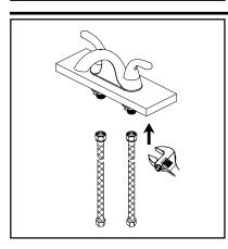
Turn on hot and cold supply valves by rotating counterclockwise.
