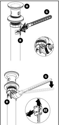
Install Pop-Up Drain Pivot Rod **G**. Insert into Drain Tailpiece **R** and rotate to tighten.
