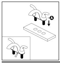
Insert the Faucet Body A through the sink deck. Apply a bead of silicone sealant around the perimeter of the Faucet Body after installation is completed and faucet is positioned as desired.
