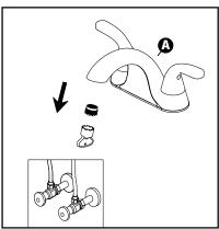
Use aerator removal tool to remove faucet aerator from Faucet Body (A). Rotate counterclockwise to loosen. Turn on hot and cold supply valves by rotating counter clockwise.
