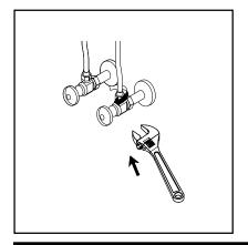
Connect hot and cold supply lines to hot and cold supply valves.
